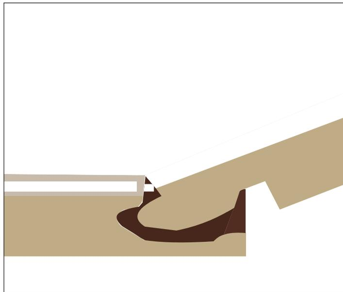
Our Click-N-Lock® Tiles come with Wel-Lock™ technology, a unique locking mechanism that obviates the need for glue or cement.
